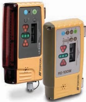
Integrated CAN support in the LS-B10W means that this system is provided with the flexibility to be used with future indicate and automatic machine control systems.
